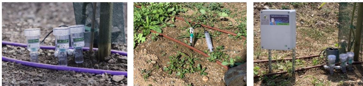
Figure 7 Tensiometers, lysimeters and iTelemeter components installed as part of the Smart Fertigation Tool.
