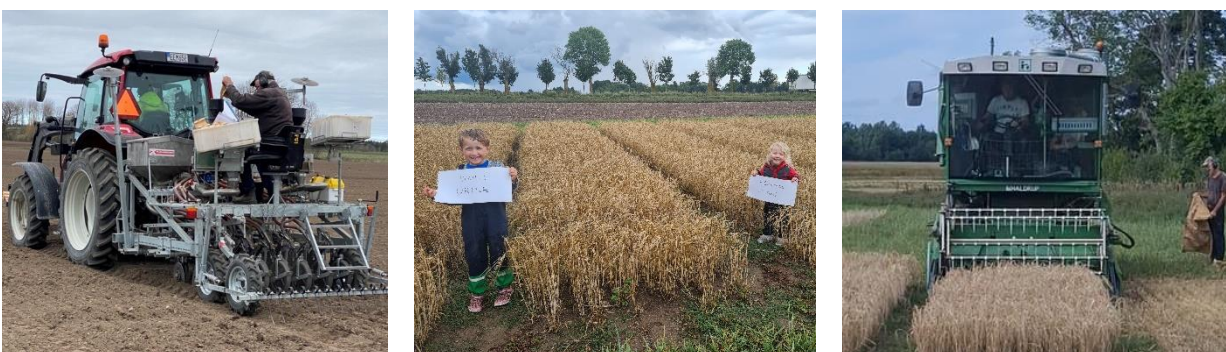
Figure 10. Farming equipment and set-up of field trials. From the left a) combi-seed drill where the barley and the urine pellets are buried into the soil 5-7 cm deep; b) visualisation of the 1.5 m wide replicates; and c) combine machinery used to harvest the barley grain.
