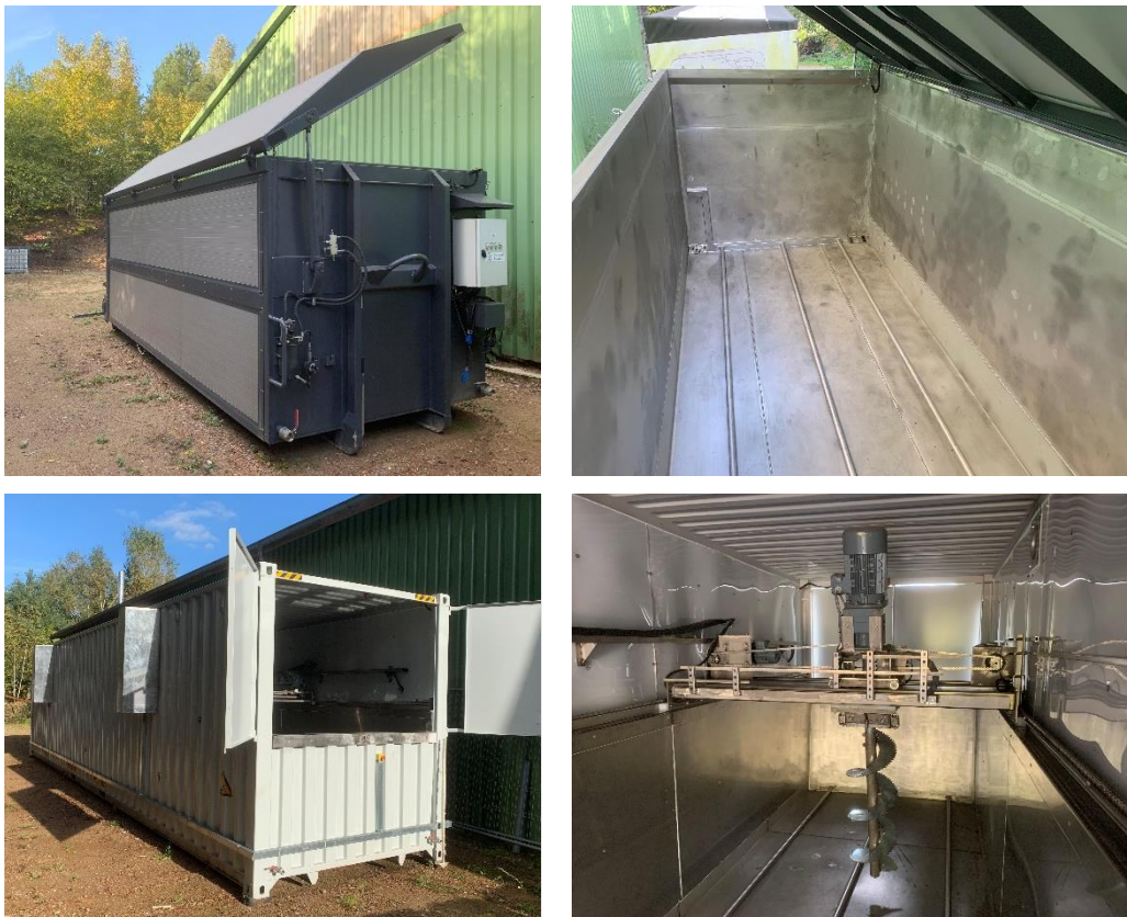
Figure 18. Top – Container system for the sanitisation of dry toilet contents by thermophilic composting (step 1). Bottom: “Earthflow” container system for De- & Recomposition of organic waste by oxygen-controlled composting (step 2)
